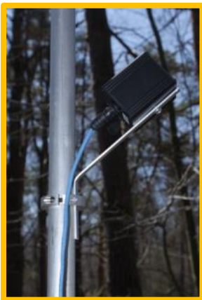
Figure 2. Standard microphone configuration for acoustic monitoring.
